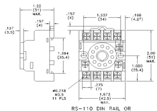
RS-110 DIN RAIL OR SURFACE MOUNT SCREW TERMINAL SOCKET
