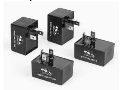
The Amperite STOP-ALERT 2 and 2M lamp pulsators are 100% solid state devices are connected in series with the third brake light of automobiles, and the stop lamp of motorcycles, to enhance awareness of stop-lamp illumination. Each time the brakes of the vehicle are applied, the stop lamp flashes rapidly for a period of 5 seconds. If the brakes continue to be applied, the stop lamp remains illuminated until the brakes are released.
